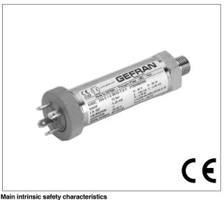
Transmitter designed and produced in compliance with Directive 94/9/CE ATEX and according to European standards for the Second group (II-surfaces), category 1, explosive atmosphere with presence of gases, fumes or mists (G) protection mode Ex ia T6, T5, T4.
