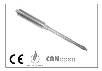
The KD Series are for use in high temperature applications where the process temperatures may reach 538°C (1000°F) such as high temperature engineered polymers. The K Series utilizes standard melt pressure principles and construction, but uses a near incompressible NAK (Sodium Potassium) for pressure transmission. The K Series strain sensing technology is bonded foil strain gage.
