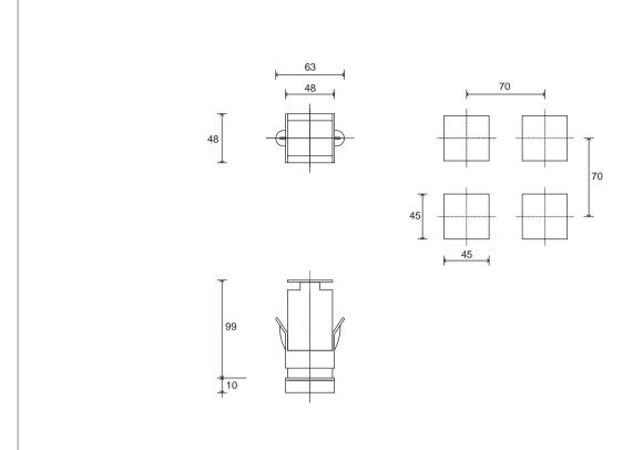
Dimensions: 48x48mm (1/16 DIN) depth 99mm
